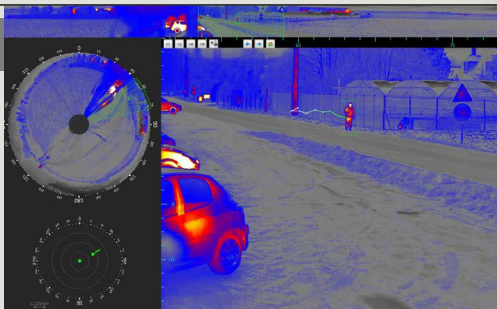
→ Infrared panoramic detection and visible identification with the same sensor
