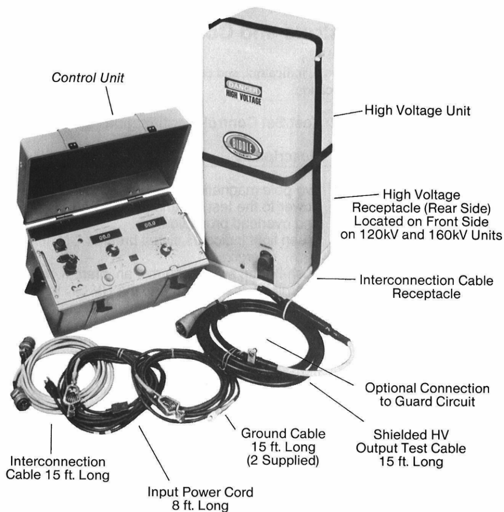
Figure 4: Test Set and Cable Identification
